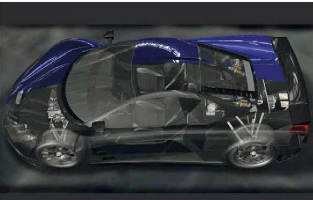
The Motion sits on a carbon-fibre composite monocoque chassis and body, F1-style double wishbone, and pushrod suspension with cast titanium uprights
