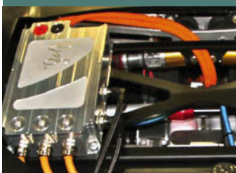
The high-voltage distribution unit inside the Kepler Motion hypercar
